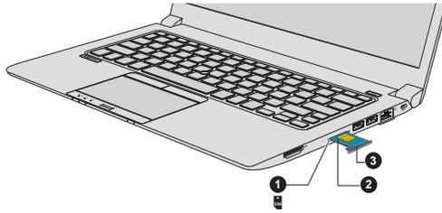
Figure 4-8 Installing the SIM Card (Z40-A)
