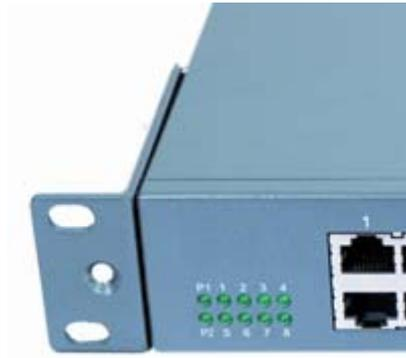
2. Install the long bracket to the other side of the device.
