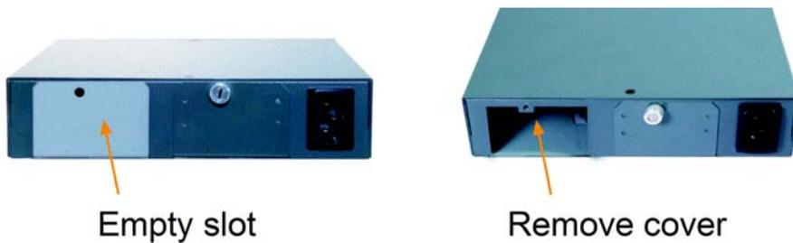
3. Install the power module into the slot until it is seated properly.
