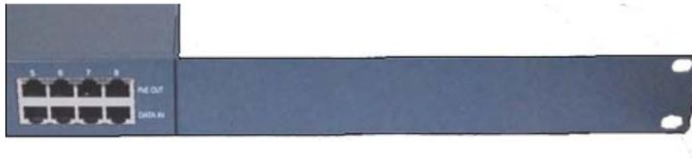
3. Mount the device in a 19" rack.
