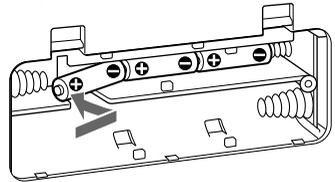
To remove the batteries, push the **+** side.
