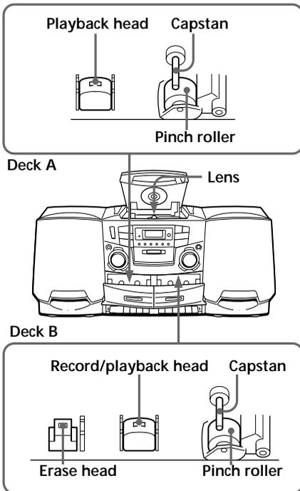
After cleaning, insert a tape when the areas cleaned are completely dry.
