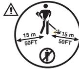
Machines fitted with saw blades or grass blades can be thrown violently to the side when the blade comes into contact with a fixed object. The blade is capable of amputating an arm or leg. Always keep people and animals at least 15 metres from the machine.
