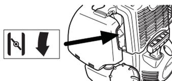
**Primer bulb:** Press the primer bulb repeatedly until fuel begins to fill the bulb. The bulb need not be completely filled.
