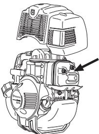
The muffler on your machine is equipped with a spark arrestor mesh, this should be cleaned regularly. A blocked mesh will cause the engine to overheat and may lead to serious damage.
