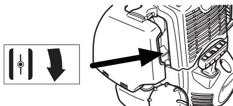
**Primer bulb:** Press the primer bulb repeatedly until fuel begins to fill the bulb. The bulb need not be completely filled.
