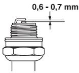
**CAUTION!** Always use the recommended spark plug type! Use of the wrong spark plug can damage the piston/cylinder. Check that the spark plug is fitted with a suppressor.
