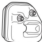
In countries that have a warm and dry climate there is a significant risk of fire. We therefore fit certain mufflers with a spark arrestor mesh. Check whether the muffler on your machine is fitted with this kind of mesh.
