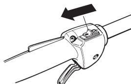
**Choke:** Put the choke in working position.
