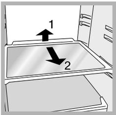
Due to the special guides the shelves are removable and the height is adjustable (see *diagram*), allowing easy storage of large containers and food. Height can be adjusted without complete removal of the shelf.
