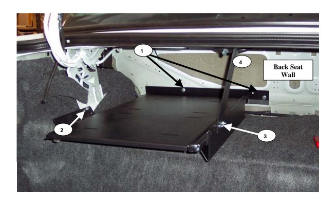
**Step 1.** Align forward radio shelf bracket with existing holes in front of trunk wall. Use 2 (two) 1/4" x 1" hex head cap screws, 2 (two) 1/4" flat washers and 2 (two) 1/4" flange nuts. Don't fully tighten bracket yet.
