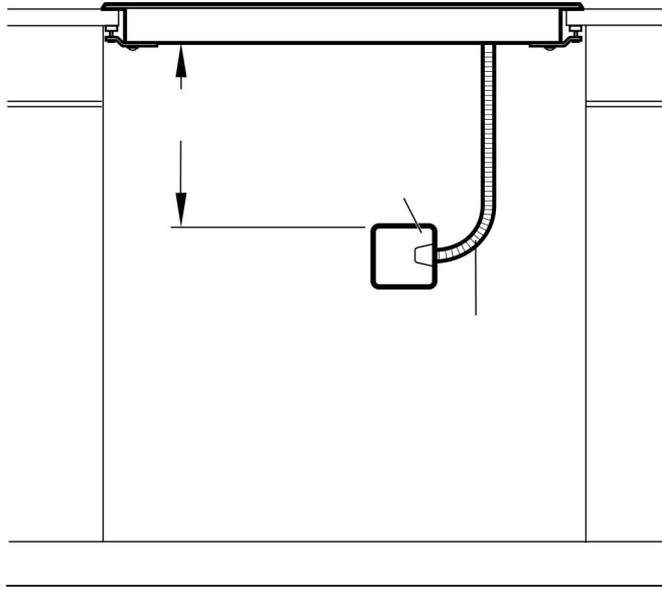
You can find the identification plate with the electrical specifications on the underside of the appliance. The junction box must be located within 3 feet of the cooktop connection. It should be easily accessible for service purposes.
