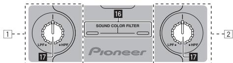
Each channel is equipped with a SOUND COLOR FILTER function by which filter effects can be achieved simply by turning a large control. The treble or bass sound can be removed by turning the [SOUND COLOR FILTER] control 17.
