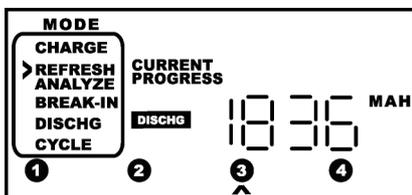
Note the charging capacity is usually higher than the actual capacity of the battery owing to some energy lost as heat. Charging capacity cannot be used to judge the performance of the battery. Instead, it can only be used to determine the progress of the charger. It is normal for this number to exceed the actual capacity by as much as 20-30%.
