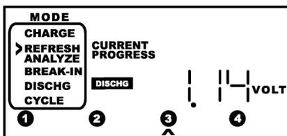
At any given time during the program, the charger will either be charging, discharging or resting. The LCD displays the action in black boxes containing **CHARGE**, **DISCHG**, or **REST**.
