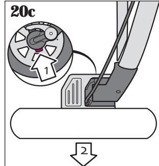
Press both front wheel release buttons to pull the front fork out of the frame tube (**Figure 20d**).
