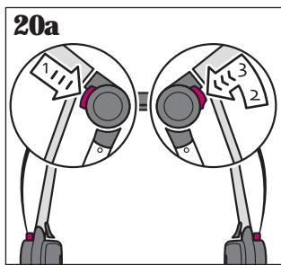
While buttons are still pressed, push the stroller down to fold toward front wheel. Push down as far as possible and secure the transport hook to prevent the stroller from unfolding during transport (**Figure 20b**). This may require some force. However, it will become easier in time.
