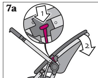
**WARNING** DO NOT use when red indicator is visible (Figures 7 & 8). DO NOT use with seat in this position.
