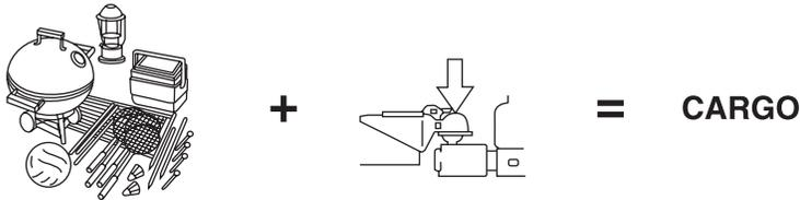
**Cargo Weight** – includes all weight added to the Base Curb Weight, including cargo and optional equipment. When towing, trailer tongue load or king pin weight is also part of cargo weight.
