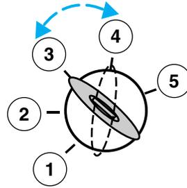
2. Turn the ignition from the 3 (OFF) position to the 4 (ON) position. Keep the ignition in the 4 (ON) position for at least one second, but no more than 10 seconds.
