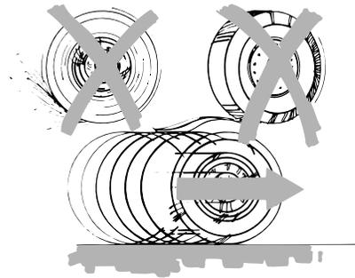
Apply the brakes steadily. Do not “pump” the brakes.
