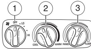
3. **Airflow control:**FLOOR directs air to the floor of the third row seating. PANEL directs air to the overhead registers of the second and third row seating. To blend the airflow, select any position between PANEL and FLOOR.
