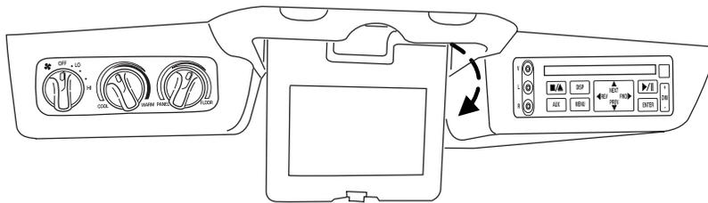
The screen rotates down to view and into the housing to store when not in use. Be sure the screen is latched into the housing when being stored.
