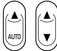
Press and hold the bottom part of the rocker switch to open the window. Press and hold the top part of the rocker switch to close the window.
