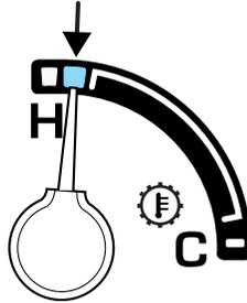
Altering the severity of the driving conditions is recommended to lower the transmission temperature into the normal range.
