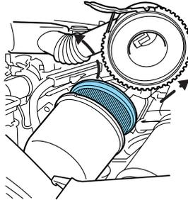
4. Install a new air filter element, ensuring the arrow on the top half of the air filter housing lines up with the notch on the bottom half of air filter housing. Be careful not to crimp the filter element edges between the air filter housing. This could cause filter damage and allow unmetered air to enter the engine if not properly seated.
