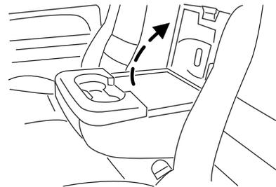
To gain access to the storage compartment in your armrest, lift the latch to open the lid. The lid cannot be opened in the upright position.
