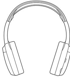
To install the batteries, lightly press down on the top of the left earpiece and slide the cover off.
