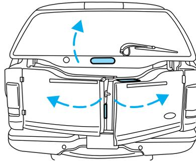
For wider loads, the cargo doors can be opened wider by unhooking the check straps from the door hinge. Make sure the check straps are reattached after loading and before closing the cargo doors..
