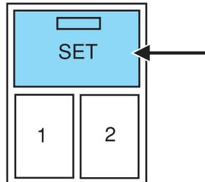
A position can only be recalled when the transmission gearshift is in Park or Neutral. A memory seat position may be programmed at any time.
