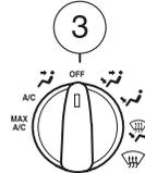
**MAX A/C:** Uses recirculated air to cool the vehicle. Air flows from the instrument panel vents only.
