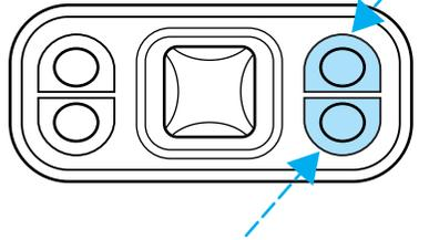
Press the control to move the seat forward, backward, up or down.
