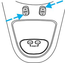
Press the ▲ portion of the VENT control to open the power rear quarter windows.
