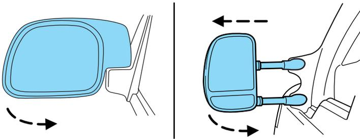
The telescoping feature (if equipped) allows the mirror to extend approximately 80 mm (3.15 inches). This feature is especially useful to the driver when towing a trailer.
