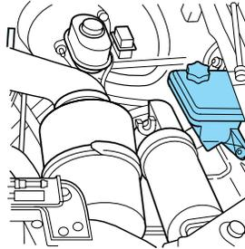
Check the fluid level when it is at ambient temperature, 20° – 80° F (-7° – 25° C):
