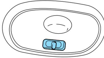
With the ignition key in the ACC or ON position, the rear dome lamp can be turned ON or OFF by sliding the control.
