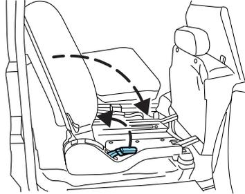
6. For bench seats only, lift up flap on seatback to release closeout panel.
