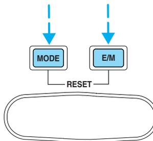
5. Release both controls. Subsequent pressing of either control will increment the zone. Press the control repeatedly until the correct zone setting for your geographic location is displayed on the trip computer.
