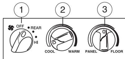
2. **Temperature control:** Determines temperature level. If the main climate control system is cooling in MAX A/C or
