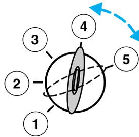
**Note:** If the engine does not start within five seconds on the first try, turn the key to 3 (OFF), wait 10 seconds and try again. If the engine still fails to start, press the accelerator to the floor and try again; this will allow the engine to crank with the fuel shut off in case the engine is flooded with fuel.
