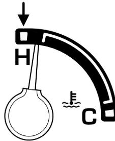
If the engine reaches a preset over-temperature condition, the engine will automatically switch to alternating cylinder operation. Each disabled cylinder acts as an air pump and cools the engine.
