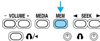
If your vehicle is equipped with an in-dash six CD player, press the MEMORY control to select the next disc in the compact disc changer. Play will begin with the first track.
