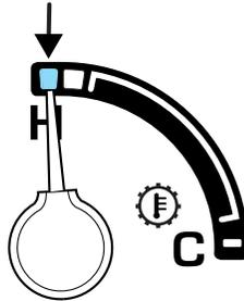
If the gauge is operating in the Yellow or Red area, stop the vehicle and verify the airflow is not restricted such as snow or debris blocking airflow through the grill. If the gauge continues to show high temperatures, see your Ford dealer.
