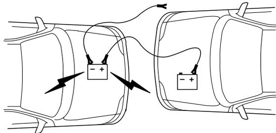
2. Remove the jumper cable on the negative (-) connection of the booster vehicle's battery.
