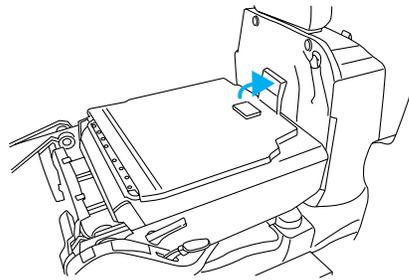
7. For bench seats only, rotate panel to closeout the space between the seatback and the floor.
