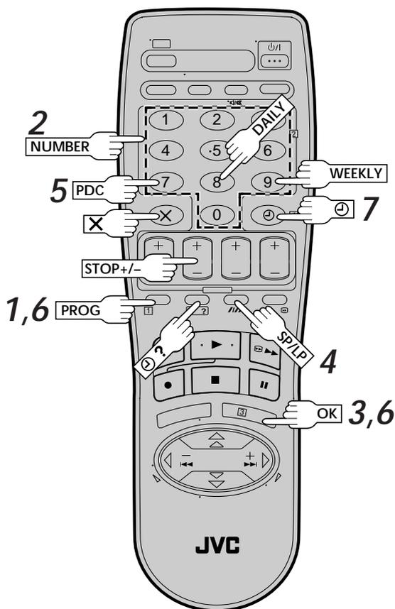
With VIDEO Plus+, timer programming is greatly simplified because each TV programme has a corresponding code number which your recorder is able to recognise.
