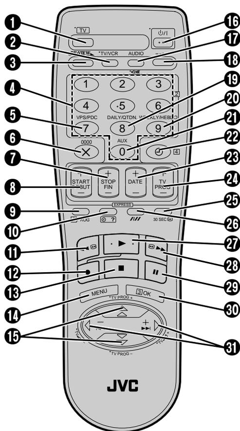
Buttons with a small dot on the left side of the name can also be used to operate your JVC TV while holding down the **TV** button.
