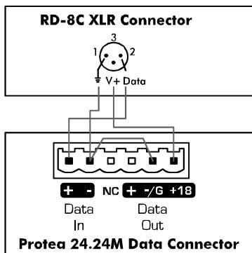
*Note: On newer 24.24M units which show an illustration of WR-5 wiring on the back panel, it is not necessary to wire pin 2 and pin 5 together at the 24.24M data connector.*
