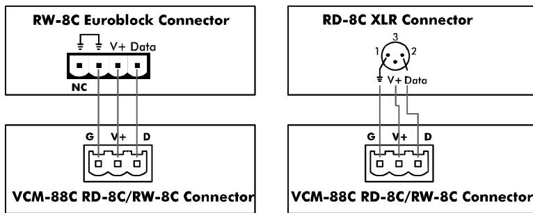
**Used with the VCM-88C,** the RD/RW-8C offers a direct correlation of remote faders to VCM-88C channels, as well as its master fader. Connect the RD-8C or RW-8C to a VCM-88C as follows:
