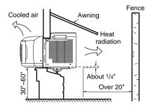
CAUTION: All side louvers of the cabinet must remain exposed to the outside of the structure.
