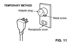
Because of potential safety hazards, we strongly discourage the use of an adapter plug. However, if you wish to use an adapter, a TEMPORARY CONNECTION may be made. Use UL-listed adapter, available from most local hardware stores (FIG. 11). The large slot in the adapter must be aligned with the large slot in the receptacle to assure a proper polarity connection.
