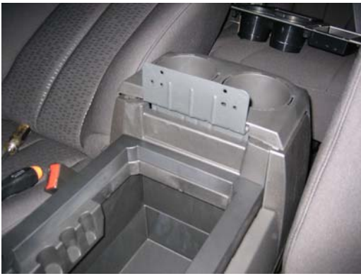
Remove (4) hex screws holding armrest pad from hinge
