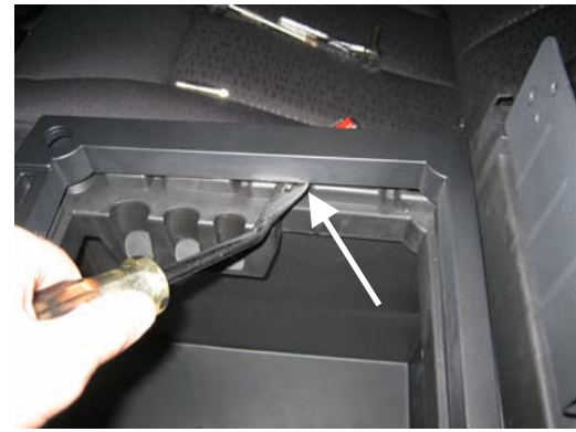
Pry up on accessory pocket trim panel and remove
