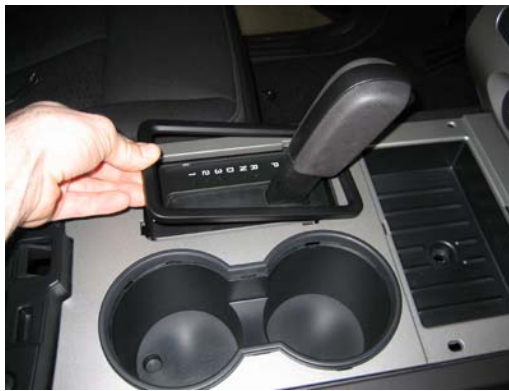
CAREFULLY remove trim from around gear shifter
