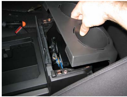
Remove the rear OEM cup holder
