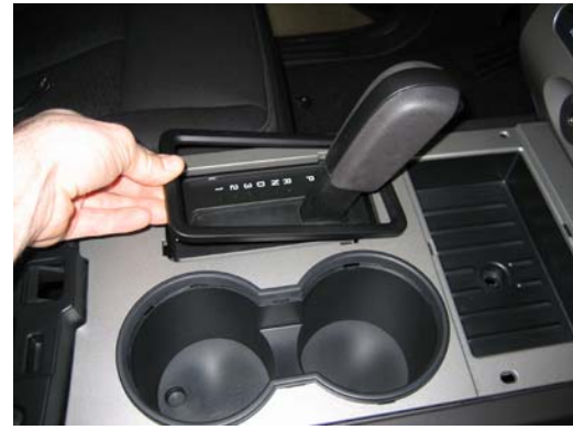
Replace the trim panel around gear shifter
