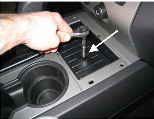
Remove hex head screw from accessory pocket
