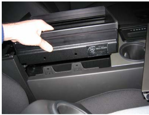
Position console so holes in side of console align w/ holes in factory console
