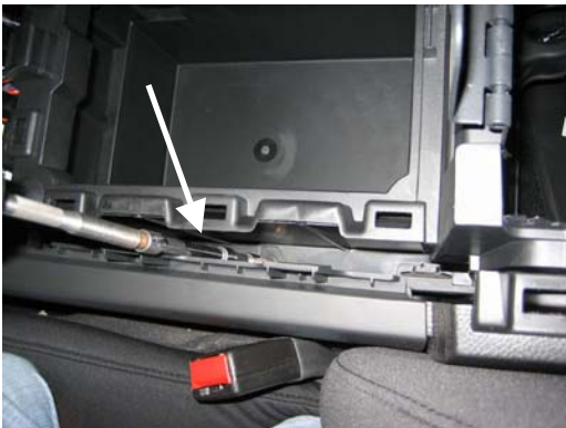
Remove hex head screws holding lower sides accessory pocket
