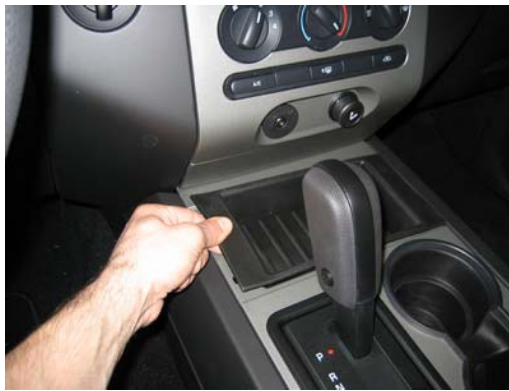
Remove accessory pocket liner as shown above
