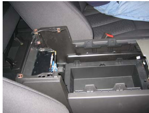
Completely remove the container of the accessory pocket
