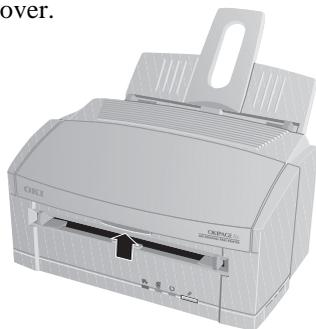
2 Remove the image drum cartridge.
