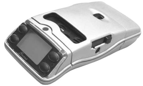
**Scott's modular pump and component assemblies will minimize downtime.** Unlike many other portable detectors, should a failure of a pump occur, the Scout® can continue to be operated with a hand aspirator or a new pump can be simply plugged in. In fact, all Scout's major components are modular and designed for simple, fast replacement in the field.
