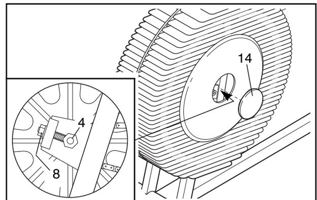
2. Pry the Access Cover (14) off the left side shield. Loosen the M8 Washer Nuts (4). To tighten the chain, turn the M6 Adjustment Nuts (8) clockwise; to loosen the chain, turn the Adjustment Nuts counterclockwise. Make sure that the fan is straight, tighten the Fan Nuts and reattach the Access Covers.
