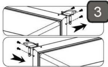
4. Remove the lower hinge and bushing from the bottom right support bracket. Remove the decorative screws from the left corner of the door and install and tighten them to the right corner holes. Remove the plastic cap from the top left corner of the door and insert it on the right top corner.
