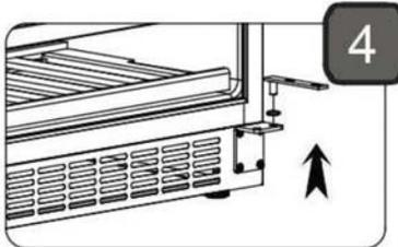
5. Install the lower hinge and bushing on the bottom left support bracket
