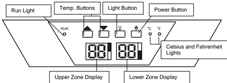
Use the up button to adjust the upper zone's temperature, and use the down button to adjust the lower zone's temperature. The temperature displayed can be in Fahrenheit or Celsius. This wine cooler has a temperature range from 41°F to 54°F for the upper zone, and 54°F to 64°F for the lower zone.
