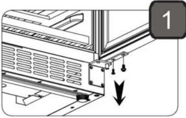
2. Carefully slide the bottom of the door forward and down, and place it on a padded surface to prevent damaging it.
