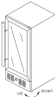
It is important for the wine refrigerator to be leveled in order to work properly. It can be raised or lowered by rotating the plastic sheaths around each of the feet on the bottom of the machine. If you find that the surface is not level, rotate the feet until the wine refrigerator becomes level. You may need to make several adjustments to level it. We recommend using a carpenter's level to check the machine.
