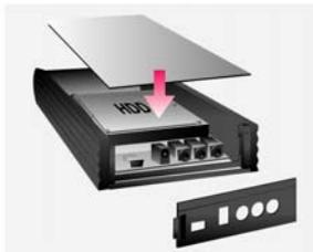
⑤ Insert the PCB into the case, and then close the top cover and front panel.
