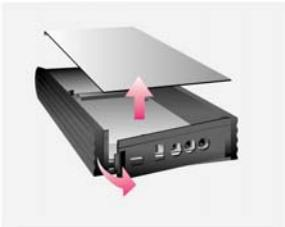
① Grip the hasp and pull back the front panel, and then open the top cover.
