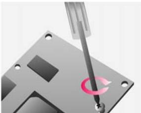
④ Screw HDD on PCB by using the supplied screws.
