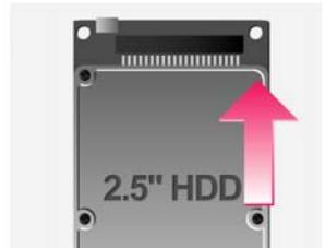
③ Grip HDD and insert it into the pins of PCB (be sure to match the 44 pins)
