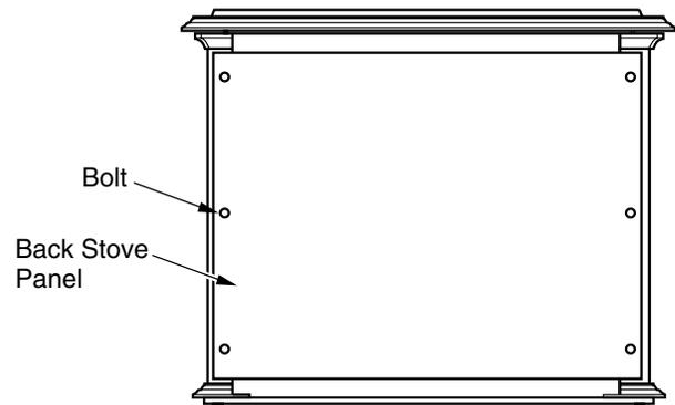
**Figure 6 - Removing Back Panel (Amity Stove Only)**
