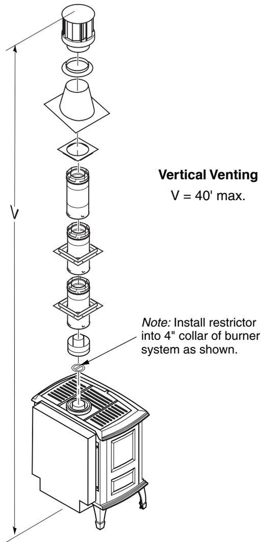
**Figure 38 - Vertical Venting Configuration With No Horizontal Run**
