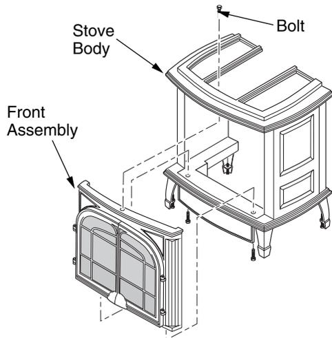
**Figure 13 - Removing Front Assembly (Oxford™ Model Shown)**
