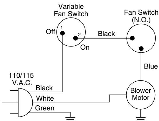
**Figure 65 - Blower Wiring Diagram for Thermostat-Controlled Models**
