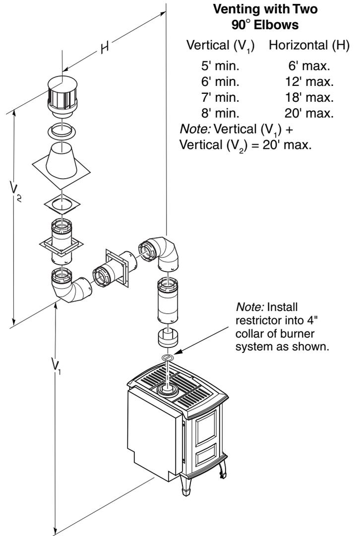
Figure 37 - Vertical Venting Configuration Using Two 90° Elbows
