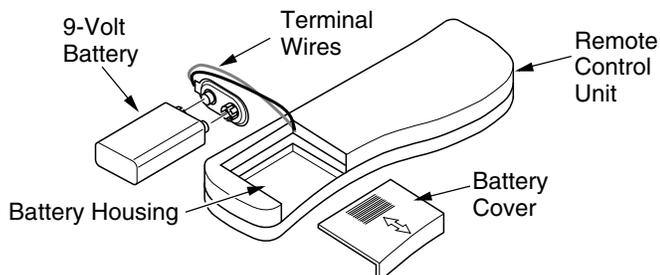
**Figure 51 - Installing Battery in Hand-Held Remote Control Unit (C)GHRCTB Series**
