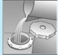
Only before using the dishwasher for the first time pour approx. 1 l / 1 1/4 pt water into the salt opening.
