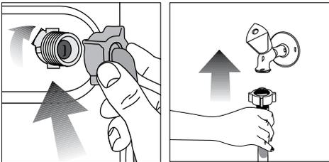
Models with double water inlets can be used as a model with a single water inlet by using a plug. Plug should be installed to the hot water valve. A rubber gasket should be used in order to prevent water leakage from the connection point.
