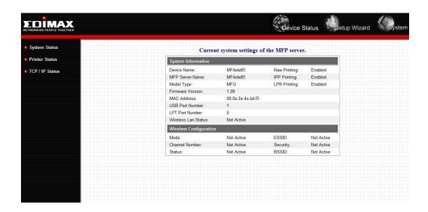
System Information includes "Device Name", "MFP Server Name", "Model Type", "Firmware Version", "MAC Address", "Wireless Configuration", and the protocols enabled status, etc.
