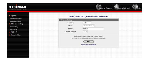
You can enable/disable the wireless function and set up the wireless parameters for the MFP Server from here. The parameters include "Function" and "ESSID". You can manually set the wireless network that you want to connect in this page or use the "Site Survey" function to automatically search for an available wireless network and associate with it.
