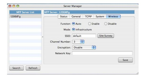
This MFP server supports WEP, WPA-PSK and WPA2-PSK security mode. If you want to use WEP encryption to protect your wireless network, you have to select "WEP". The wireless security setting should match other wireless devices in the same network.
