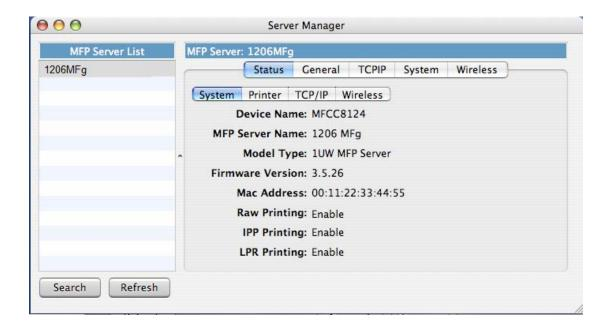
To run the "Server Manager" configuration utility, click the "Search" button. The configuration utility will delay for several seconds because the utility is using the system's available network protocols to search for all MFP Servers on the network. All available MFP Servers will be listed under "MFP Server List" on the left side of the window.
