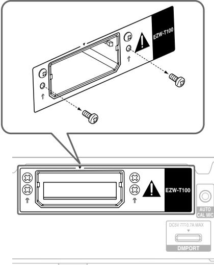
3 Use the screws that you removed from step 1 to fasten the wireless transmitter.
