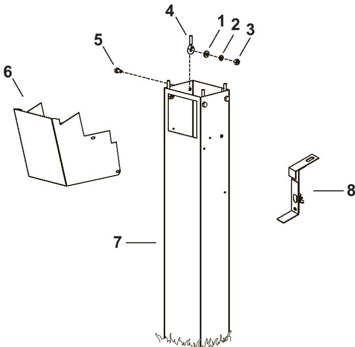
**REMOVE PROTECTIVE COATING FROM STAINLESS STEEL PARTS STARTING AT POP RIVETS AND VERIFY THAT ALL PARTS LISTED IN THE EXPLODED VIEW ON THIS PAGE HAVE BEEN INCLUDED BEFORE BEGINNING THIS INSTALLATION.**
