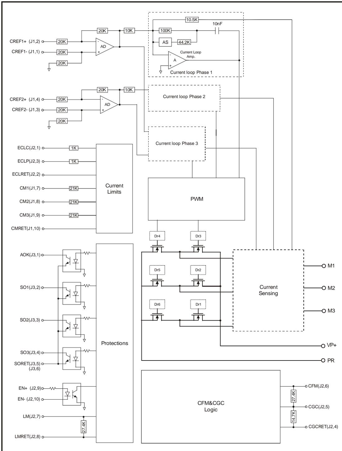
Figure 2-1: Raven Block Diagram
