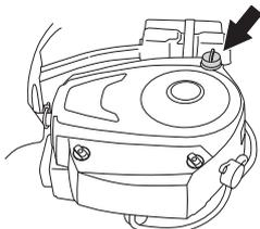
The dipstick should be **completely screwed down**
