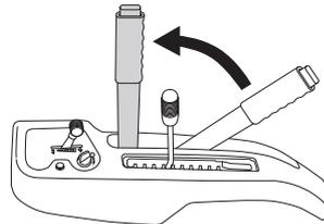
If the lock button is pressed in and the lever is moved forwards the unit will be lowered and the blades will automatically start to rotate (mowing position).
