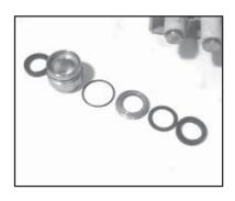
7. Remove the weep return ring (25), pressure ring (24), and v-sleeve (23) from the valve casing (26). Remove the v-sleeve (23A) from the seal case (20). Inspect all parts, including o-ring (21) for wear and replace as
