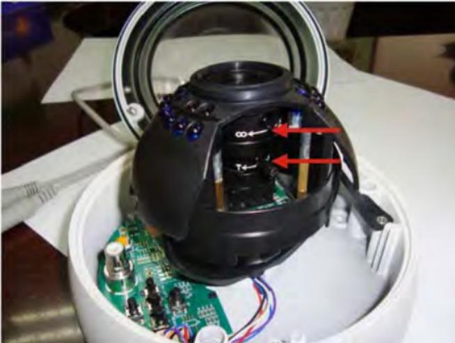
9. Top screw adjusts focus, bottom screw adjusts lens size.
