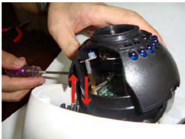
7. Loosen the screws on both sides with a screwdriver
