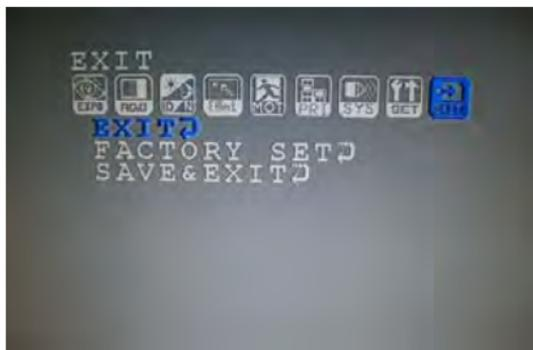
When all settings are complete, press "Up", "Down" to move the cursor to "Return", then press "OK", "Exit" dialog will appear, select "Exit "(Exit menu, do not save the settings of parameters) or "factory original settings" (it means to return to factory settings ) or "Save & Exit" (save the changes to parameters and then exit the menu) and then press "OK" to perform the corresponding return functions.
