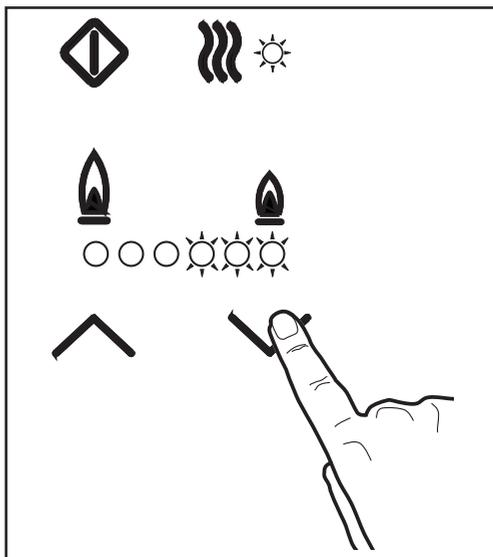
After 60 seconds, you can remove the safety device on the burner by touching both the Increasing Controls
