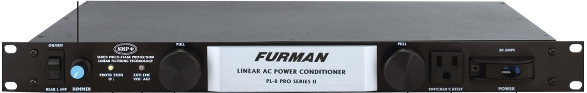
Rear light switch    Dimmer control for front rack lights    Protection OK & Extreme Voltage LED's    LED Rack Lights    Switched Outlet    Power Switch
