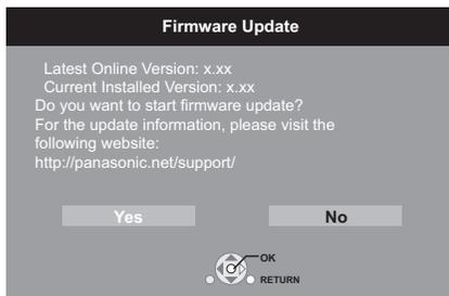
**DO NOT DISCONNECT** the unit from the AC power or perform any operation while the update takes place. After the firmware is installed, “FINISH” will be displayed on the unit’s display. Unit will restart and the following screen will be displayed.
