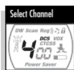
2. Press the MODE button until the Dual Watch icon and the channel number flash on the display.
