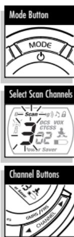
While setting channel scan, if you do not press any buttons for 15 seconds your radio will automatically return to LISTENING MODE on the channel or channel/privacy code displayed before you entered Mode Functions.
