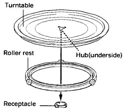
1. Place the roller rest on the cavity bottom.
