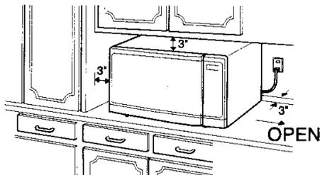
A minimum clearance of 3 inches is required between the oven and any adjacent wall. One side must be open.
