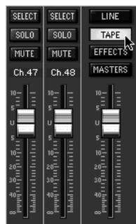
2. Turn off the L-R assignments for channels 25–30 (tracks 1–6 returns). Turn off the L-R assignments for any other channels you don't want to monitor while bouncing down.
