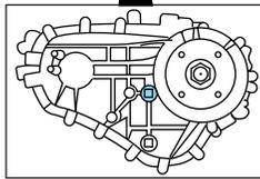
3. Add only enough fluid through the filler opening so that the fluid level is at the bottom of the opening.
