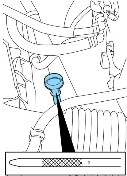
6. Wipe the indicator clean. Insert the indicator fully, then remove it again.
