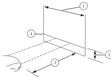
3. Turn on the low beam headlamps to illuminate the wall or screen and open the hood. Cover one of the headlamps so no light from that lamp hits the wall.
