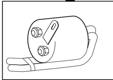
TorqShift-equipped vehicles which do not have the externally mounted filter will have the transmission fluid filter located inside the transmission bottom pan. Refer to the *scheduled maintenance information* for service intervals for automatic transmission fluid and each transmission filter type. See your authorized dealer for replacement.
