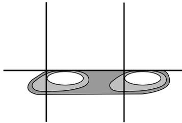
5. Locate the vertical adjuster (2) for each headlamp. Adjust the aim by turning the adjuster control either clockwise (to adjust up) or counterclockwise (to adjust down).
