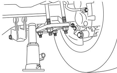
13. Insert the jack handle into the pump linkage.
