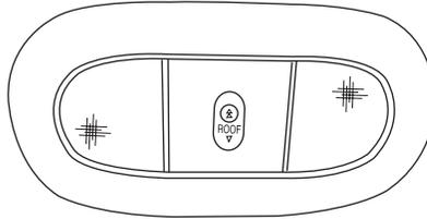
**To close the moon roof:** Press and hold the ▼ control until the glass panel stops at the “comfort” position. Press and hold the control again until the glass stops moving (the moon roof does not go to the comfort position). When fully closed, the rear portion of the glass panel will appear higher than the front portion.
