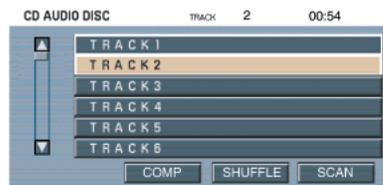
**COMP (Compression):** Compression brings soft and loud CD passages together for a more consistent listening level when in CD mode. Press to turn the feature ON/OFF
