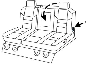
**To flip the seat cushion up,** pull up on the lever located on the side of the seat cushion to rotate the cushion up until it locks into a vertical storage position, gaining access to the grocery hook located on the underside of the driver-side seat cushion. The maximum load is 25 lb. (11 kg).
