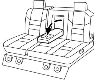
To gain access to the 60/40 load floor, store the cushion in the upright locked position. Pull up on the straps located at the sides of the load floor, and rotate forward until resting on the carpet.
