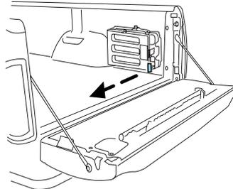
2. Rotate the storage hinge rearward to unlatch the panels.
