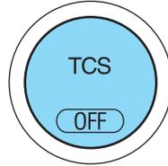
If you should become stuck in snow or ice or on a very slippery road surface, try switching the Traction Control<sup>®</sup> system off. This may allow excess wheel spin to “dig” the vehicle out and enable a successful “rocking” maneuver.
