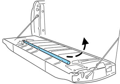
3. Rotate the center molding to unlatch the tailgate.
