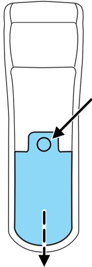
Batteries are supplied with the remote control unit. Since all batteries have a limited shelf life, replace them when the unit fails to control the DVD player.
