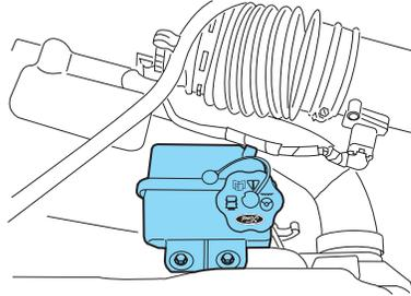
Check the fluid level when it is at ambient temperature, 20°F–80°F (-7°C–25°C):
