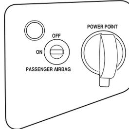
**On SuperCab and Crew Cab models,** another power point is located on the rear of the center console (if equipped).
