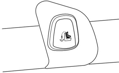
6. Clip the tether strap to the anchor as shown.
