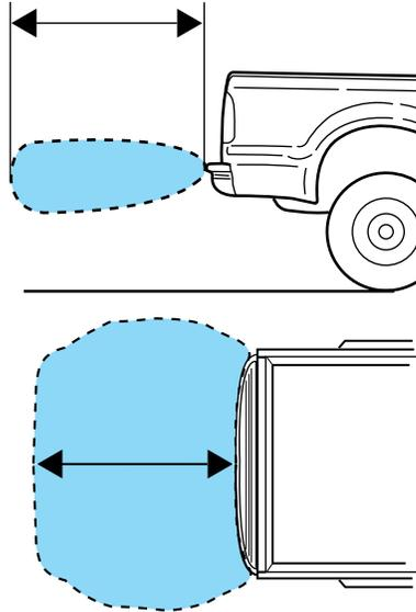
The RSS may have reduced performance or an increased chance of false detection if the tailgate is not locked and in the upright position. If the tailgate is down, the RSS tone may be heard intermittently or continuously. The tone may also be heard if items in the truck bed protrude rearward outside the bed.
