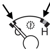
**Yellow area** (warning) — the transmission fluid is higher than normal operating temperature. This can be caused by special operation conditions (i.e. snowplowing, towing or off road use). Refer to *Special Operating Conditions* in the *scheduled maintenance information* for instructions. Operating the transmission for extended periods of time with the gauge in the yellow area may cause internal transmission damage.
