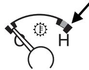
If the gauge is operating in the Yellow or Red area, stop the vehicle and verify the airflow is not restricted such as snow or debris blocking airflow through the grill. If the gauge continues to show high temperatures, see your authorized dealer.
