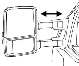
If equipped with power telescoping mirrors, you can simultaneously position both mirrors using the power telescope switch found on the door trim panel.
