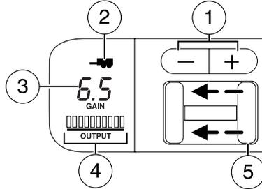
2. **Trailer connection indicator:** This lamp indicates trailer electrical connection status.
