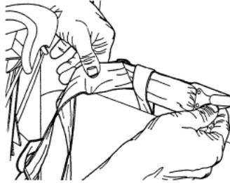
2. Attach the strap hook onto the loop behind an adjacent seating position.
