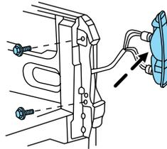
2. Remove the two bolts from the tail lamp assembly and carefully pull the lamp assembly from the tailgate pillar by releasing the two retaining tabs.
