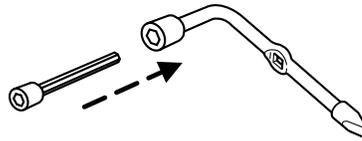
2. Attach the spare tire lock key (A) to the jack handle (B).
