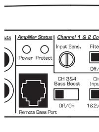
1) **CH 3&4 Bass Boost:** This switch allows the user to activate a 6 dB boost centered at 48 Hz for channels 3&4. When the “CH 3&4 Bass Boost” is activated, the inputs to “CH 3 (Left)” and “CH 4 (Right)” are summed to create a mono signal. The “Filter Mode” switch in the “Channel 3 & 4” section must be in the “LP” position for the bass boost to be functional.
