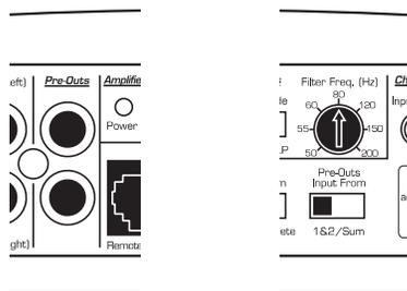
1) **“1&2”:** In this mode, the preamp output delivers the same signal that is connected to the e4300’s “CH 1 (Left)” and “CH 2 (Right)” Inputs. This mode is useful for feeding a subwoofer amplifier when the e4300 is being used to drive front and rear speaker systems. This preamp output mode will track the signal level of channels 1&2, allowing fading of the rear channels without affecting the subwoofer level.
