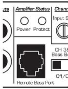
1) **“Power” (Green):** lights to indicate that the amplifier is turned on and operating normally.
