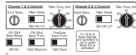
**1) "Filter Mode" Control:** The e4300 employs a 12dB per octave filter for each pair of channels (one filter for channels 1&2 and another filter for channels 3&4). Each of these filters can be configured independently into one of two filter types or defeated completely by way of the three-position "Filter Mode" switches:
