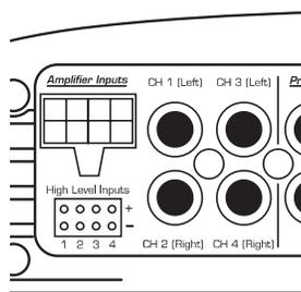
If you wish to send four discrete channels into the e4300, simply use all four inputs (channels 1 & 2 and channels 3 & 4) and set the "CH 3&4 Input From" switch to "Discrete".
