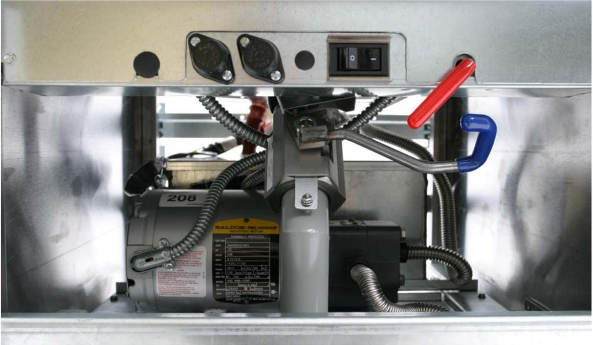
The blue handle drains the frypot. The red handle operates the filter pump.
