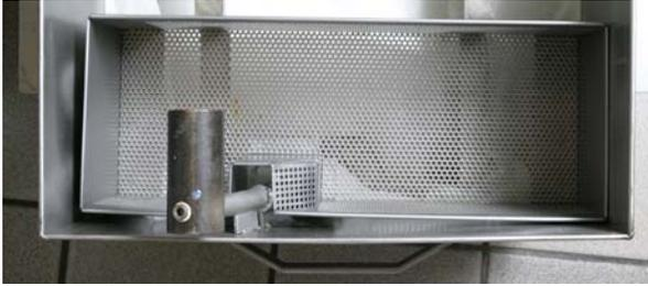
Empty the filter pan crumb tray into a fire-proof container at the end of frying operations each day. **DO NOT ALLOW CRUMBS TO ACCUMULATE IN TRAY.**
