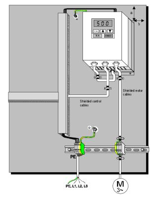
Figure: Hitachi frequency inverter with footprint filter
