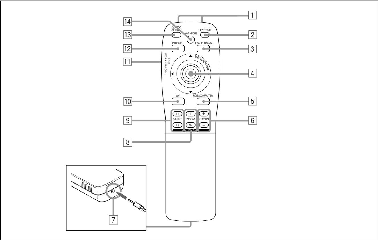
**1 Remote control's signal transmitter**
