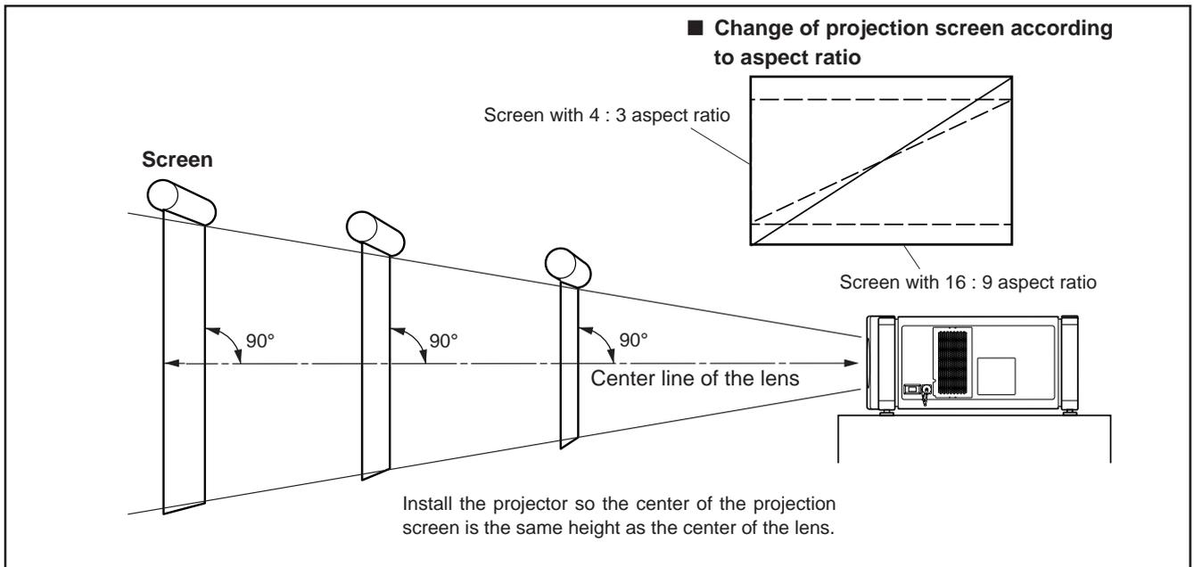
The separately sold lenses used on the projector have a lens shift function. With the lens used, you can adjust the projected image vertically using the setting menu or the remote control's SHIFT button U or D.
