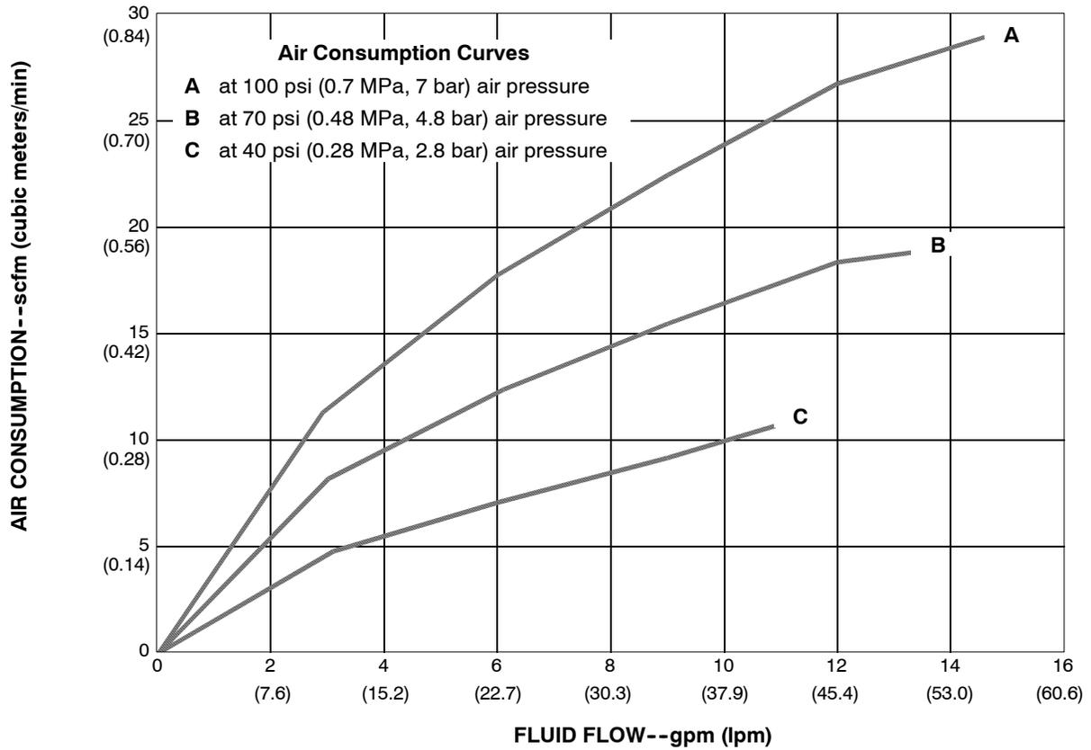
**To find Pump Air Consumption** (scfm or m<sup>3</sup>/min) at a specific fluid flow (gpm/lpm) and air pressure (psi/MPa/bar):
