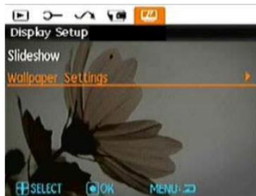
2. Press the
