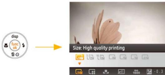
2. Press the Down button to enter the advanced functions selection screen, press Left/Right button to select the function that you want to set.
