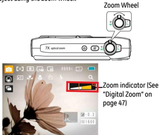
Optical zoom is initially used until it reaches the maximal threshold. Thereafter, it will switch over from optical to digital zoom. After adjusting, the zoom axis display will be hidden, only **T**
