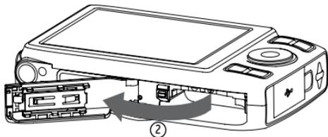
2. Insert the battery into the battery slot in the correct position as shown in the following diagram.
