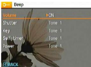
3. Press the
