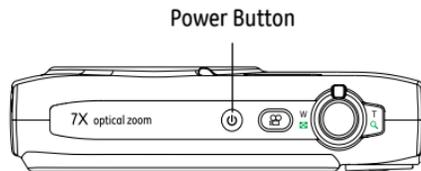
When the camera is turned on, it will be at the same shooting mode based on the last use. You can turn the Mode Dial on the top to select. When using the camera for the first-time, the language setting page will appear.
