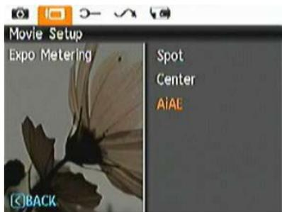
3. Press the Up/Down button to select an option or the Left or menu button to return to the menu.
