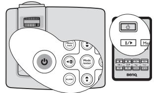
**!** If the projector is still hot from previous activity, it will run the cooling fan for approximately 90 seconds before energizing the lamp.
