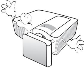
8. The lamp becomes extremely hot during operation. Allow the projector to cool for approximately 45 minutes prior to removing the lamp assembly for replacement.
