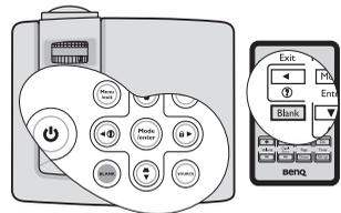
You can set the blank time in the **SYSTEM SETUP: Basic > Blank Timer** menu to let the projector return the image automatically after a period of time when there is no action taken on the blank screen. The length of time can be set from 5 to 30 minutes in 5-minute increments.
