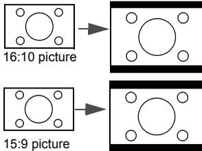
3. **4:3:** Scales an image so that it is displayed in the center of the screen with a 4:3 aspect ratio. This is most suitable for 4:3 images like computer monitors, standard definition TV and 4:3 aspect DVD movies, as it displays them without aspect alteration.
