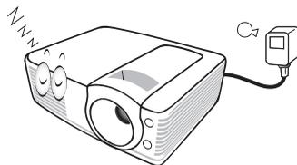
6. When the projector is under operation, you may sense some heated air and odor from its ventilation grill. It is a normal phenomenon and not a product defect.
