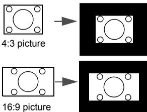
4. **16:9:** Scales an image so that it is displayed in the center of the screen with a 16:9 aspect ratio. This is most suitable for images which are already in a 16:9 aspect, like high definition TV, as it displays them without aspect alteration.
