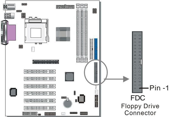
The system supports 5 possible floppy drive types: 720 KB, 1.2 MB, 1.44 MB, 2.88 MB, and LS-120. In addition, this Motherboard supports a 3-mode (720KB/1.2MB/1.44MB) floppy commonly used in Japan. Connect one side of the 34-pin flat cable to the floppy drive and plug the other end to the floppy drive connector on the Motherboard. This Motherboard can support up to 2 floppy drives.
