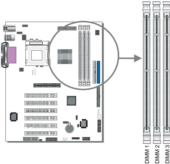
Your board comes with two DIMM sockets, providing support for up to 512MB of main memory using unbuffered and Non-ECC DIMM modules from 32MB to 512MB, No registered DIMM support. ***Supports up to 3 Double sided DIMMs at 100MHz system memory. Supports up to 2 double sided or 3 single sided DIMMs at 133MHz system memory bus.***
