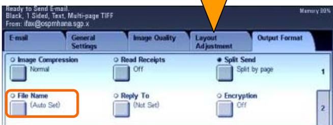
5 On the [Output Format] tab, select 'File Name' or 'Split Send' if necessary. Press the <Start> button.
