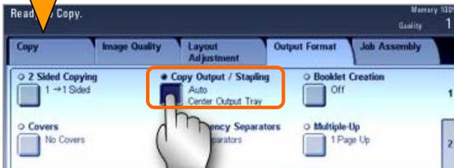
2 Select [Copy Output] in [Copy] tab; or select [Output Format] tab, select [Copy Output / Stapling].
