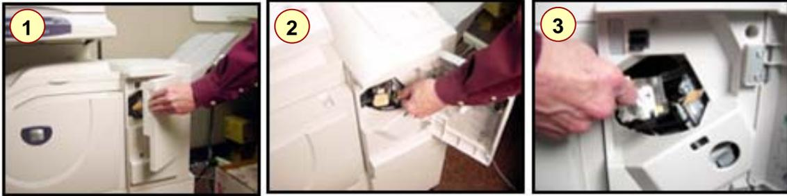
**NOTE:** The staple case contains approximately 5,000 staples. A message will be displayed on the Touch Screen when the machine runs out of staples. Make sure to have a replacement staple case available.
