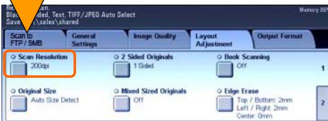
4 Select [Layout Adjustment] tab - 'Scan Resolution' if necessary.
