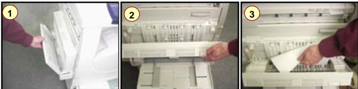
1. Open Paper Tray 5 (Bypass Tray), which is located on the left side of the machine.
