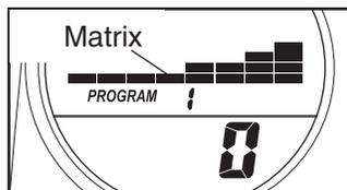
When a preset program is selected, a matrix in the left display will show the first eight resistance settings of the program (see the drawing above). The right display will show how long the program will last.
