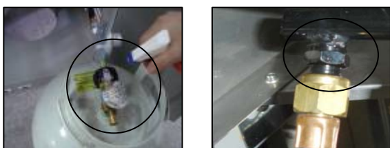
Gas Connection Leak Check
