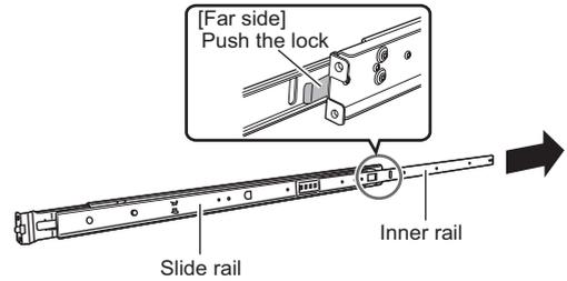
4 Attach the inner rails on the right and left side of the server.
