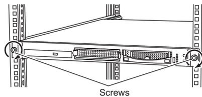
If the server or peripheral devices are not installed, install the attached blank panel to the rack.
