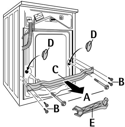
**Attention!** Push in the plug caps so firmly that they engage in the rear panel (this protects the inside of the unit against splash water).
