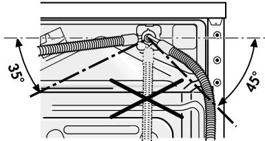
2. Connect the hose with the straight connection to a water tap with a screw thread of R 3/4 (inches).
