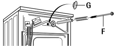
**Attention!** Push in the plug cap so firmly that it engages in the rear panel (this protects the inside of the unit against splash water).
