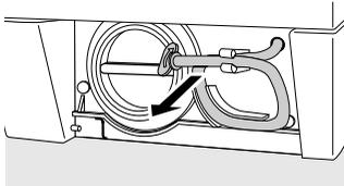
**4.** Place the collecting vessel underneath.
